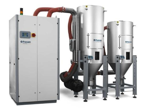
Double desiccant tower models, with an airflow rate from 200 to 800 m<sup>3</sup>/h, supply air at a dew point lower than –55°C. The process air temperature can be set up to 150°C (200°C for the HT version). The DP 619 - DP 624 Dry-
